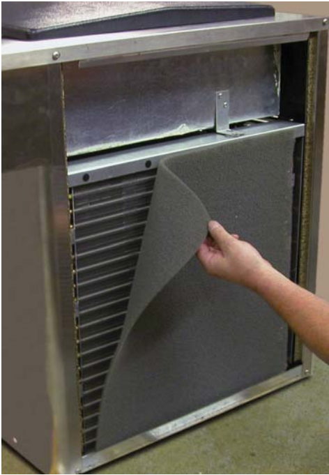
Figure 3-8 F122 Condenser Filter Removal
