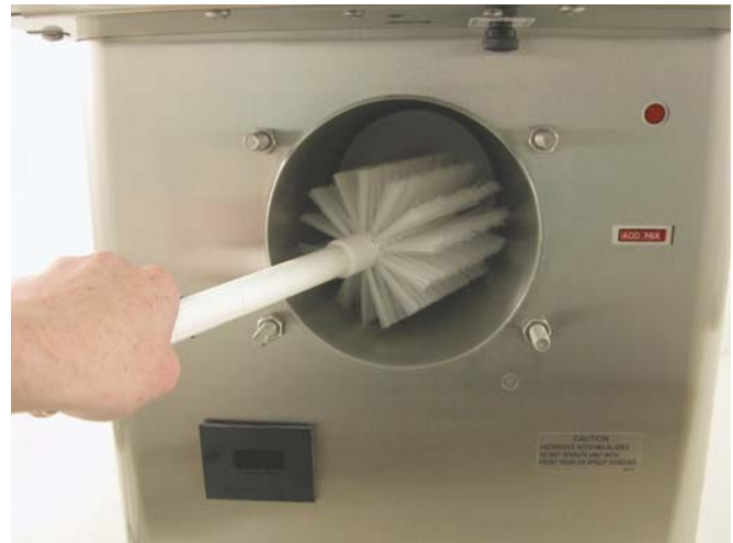
Figure 3-7 Cleaning Freezing Cylinder
