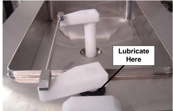
**Figure 3-9 Flow Control Arm Lubrication**
