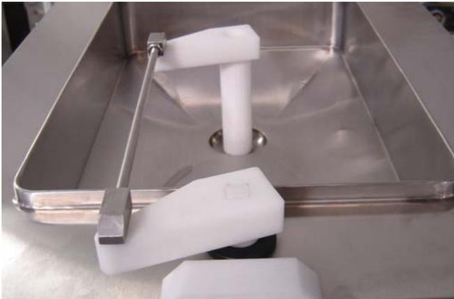
**Figure 3-3 Flow Control Assembly**
