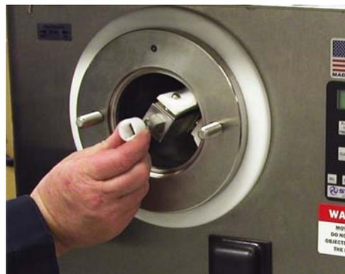
**Figure 3-7 Install Front Wear Bushing**
