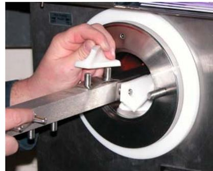
**Figure 3-6 Installing Auger Blades**
