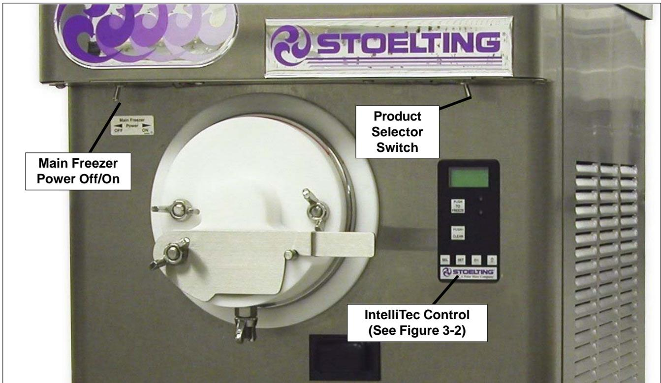
Figure 3-1 Machine Controls
