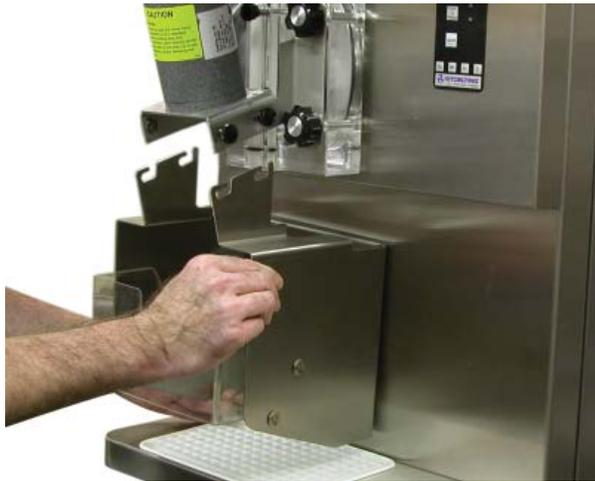
Figure 3-3 Removing Splash Shield Bracket
