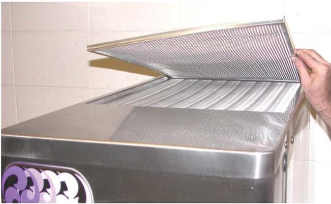
**Figure 4-4 Removing Condenser Filter**
