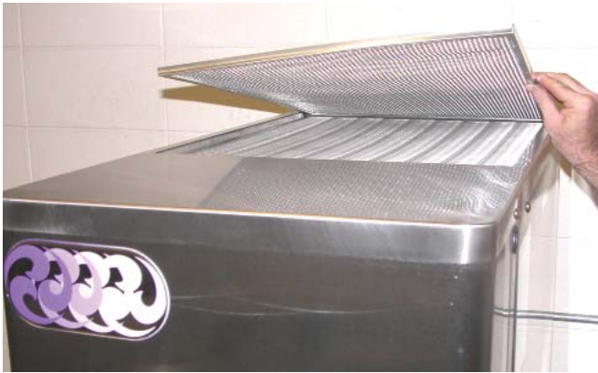
Figure 4-4 Removing Condenser Filter
