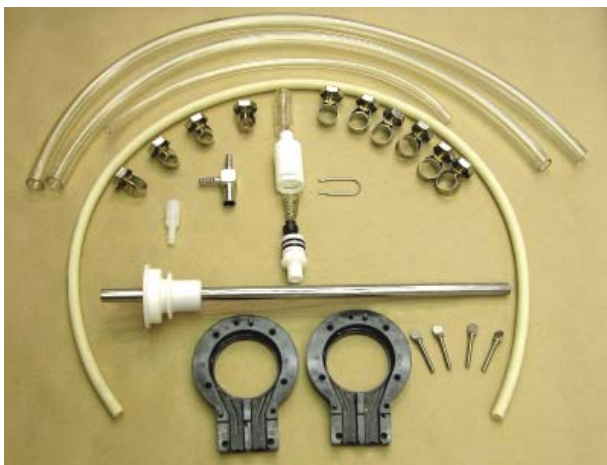
Figure 3-10 Mix Pump Removable Parts
