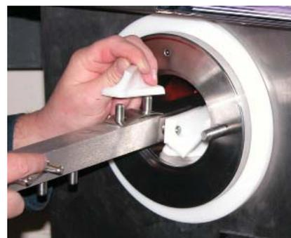
**Figure 3-6 Installing Auger Blades**
