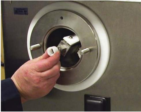
**Figure 3-7 Install Front Wear Bushing**
