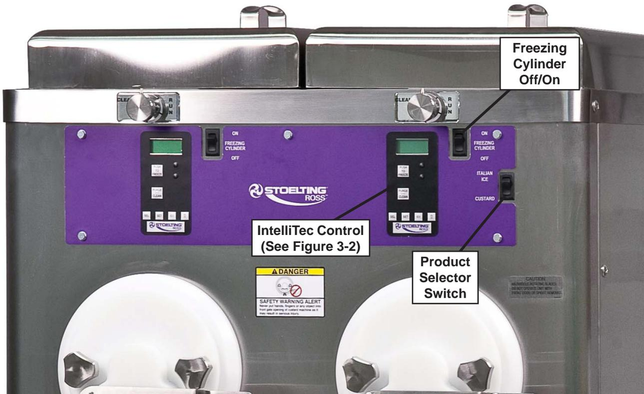
Figure 3-1 Machine Controls
