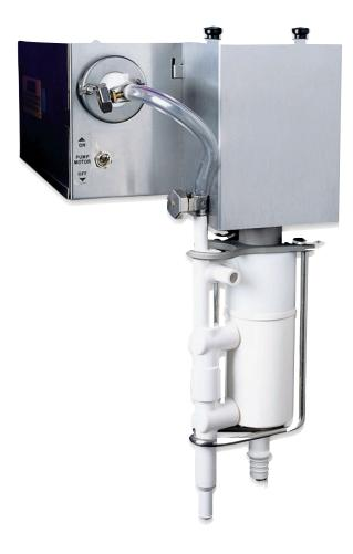
The 219 pump has a capacity of 45 gallons per hour of standard soft serve or shake mix with an adjustable overrun. For use with all Stoelting manufactured freezers. Includes a built-in pressure relief valve to prevent excessive pressure build-up in the freezing cylinder or mix line, and air-controlled pressure switch and overload protection. Factory set pressure.
