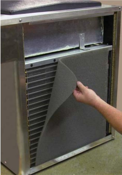
**Figure 3-8 F122 Condenser Filter Removal**
