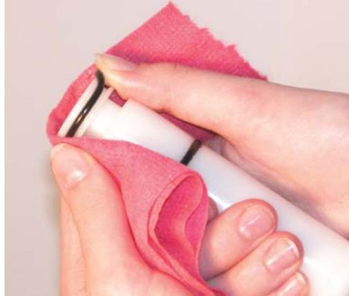
**Figure 3-4 Removing O-Ring**
