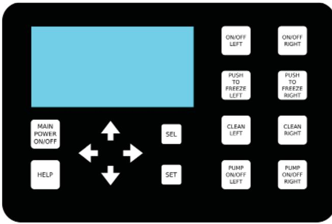
Figure 3-2 IntelliTec2 Control
