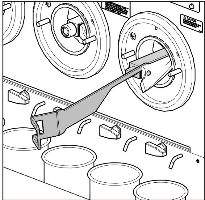
**Figure 3-15 Removing Auger**
