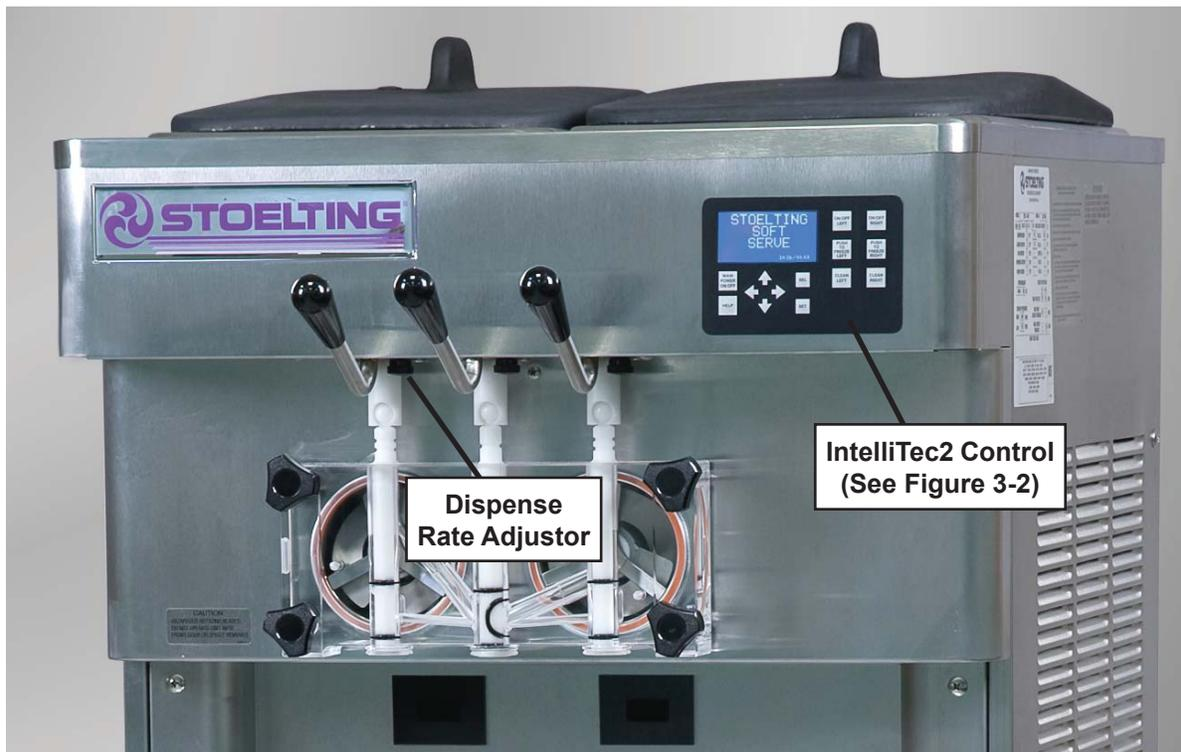
Figure 3-1 Machine Controls
