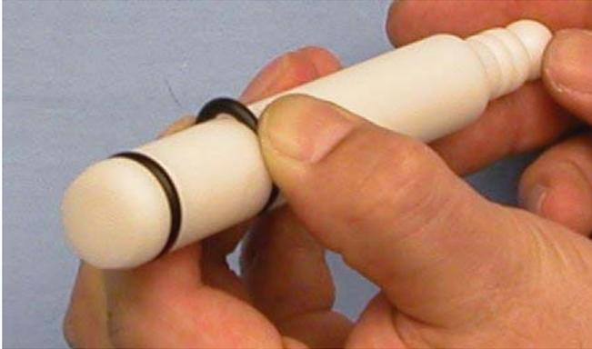
Figure 3-4 Removing O-Ring
